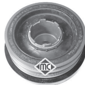
05723 Ø173 mm - 6+4canales series 1-3-5 E87/E90/E46/E60/X3 1.8D-2.0D, r.o. 11237801977-11237793882
