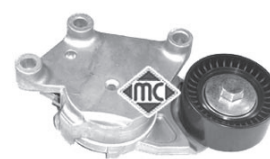
05422 tensor correa alternador 1.4 HDi eco 70 - 1.6 HDi 110 206 oe: 1611425680 -5751.H6
