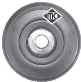
04734 Ø 151/155 mm - 7 canales motor 1.9 Diesel - DTi F9Q MEGANE II - MASTER II - SPACE r.o. 820045775
